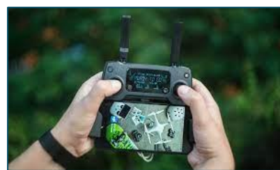
Figure 1 - Operating a UAS using a proprietary app to stream full motion video to a mobile phone.
