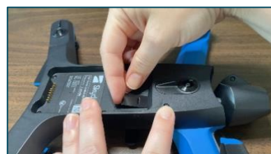
UAS operator installing the micro-SD cards to store high resolution photos and video taken during flight.
