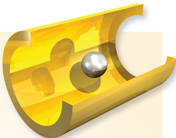
A cut-away rendering of a Nova hohlraum geometry created by the code.
