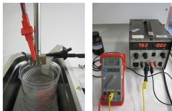
Fig. 2: Plating setup in Target Fabrication.
