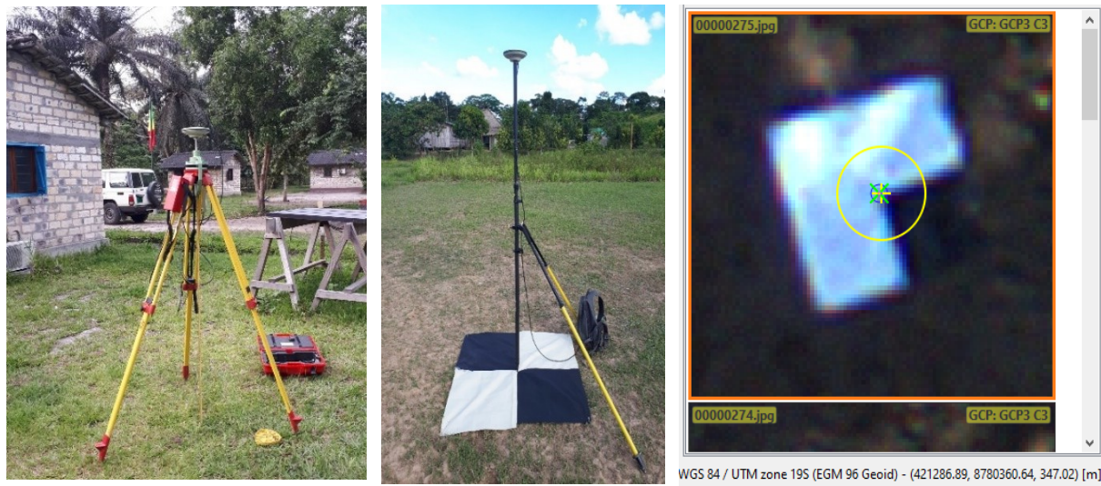
Figure 3 – Example of the base station set up (in the village of Epena, Republic of Congo; Loan 1109) (Left), the data from which is used to correct the UAV flight trajectory, and the data collected from the rover receiver, which was used to collect GCPs (centre; example from Peru under Loan 1109). These GCPs were clearly visible in the RGB images (right image) and the LiDAR data. The estimated position is identified with a blue dot. The distance to the centre of the target (defined manually) was 0.01, 0.01, 0.01 (x,y,z).
