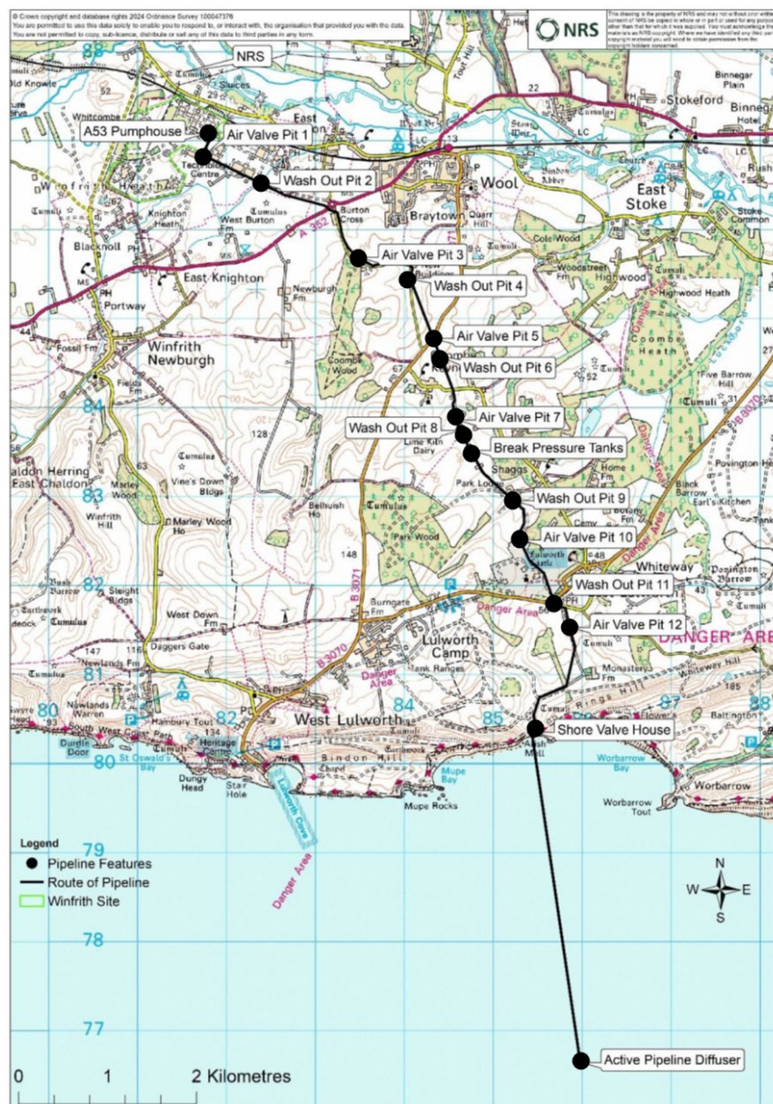
Figure 8 – Route of the Sea Discharge Pipeline from the Winfrith Site to Shore Valve House
