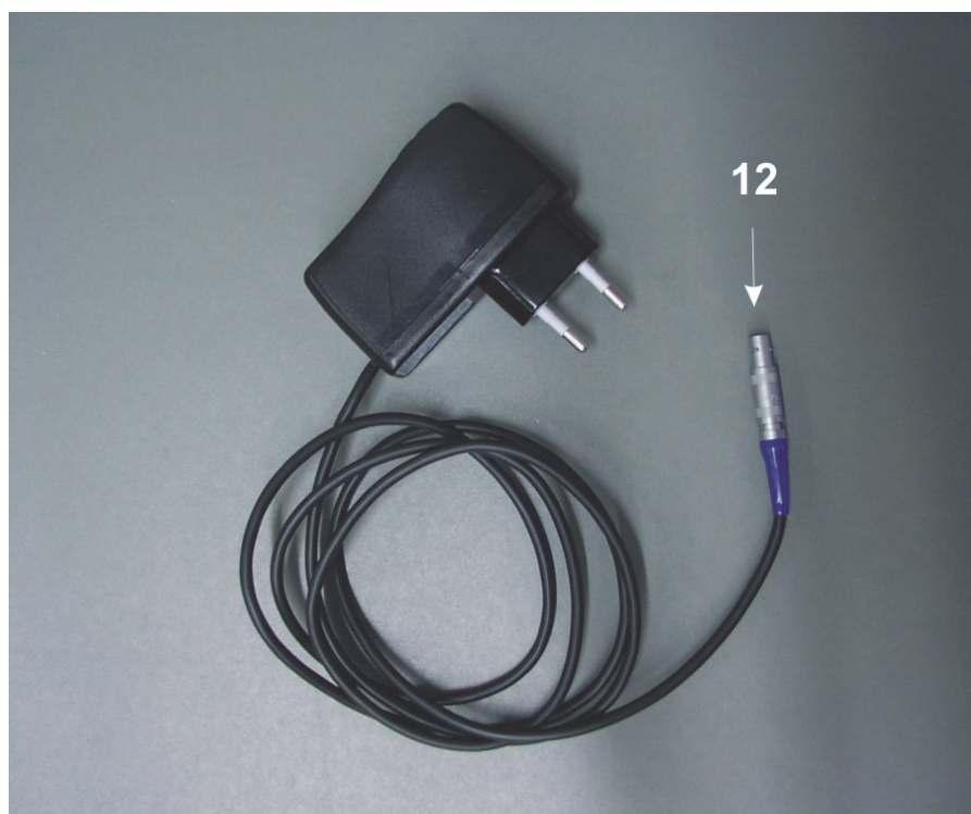
Fig. 6 External power supply for the AIOSAP module. The power supply operates on 110 V - 230 V AC. The switch on the power supply has to be set to 6 V.
