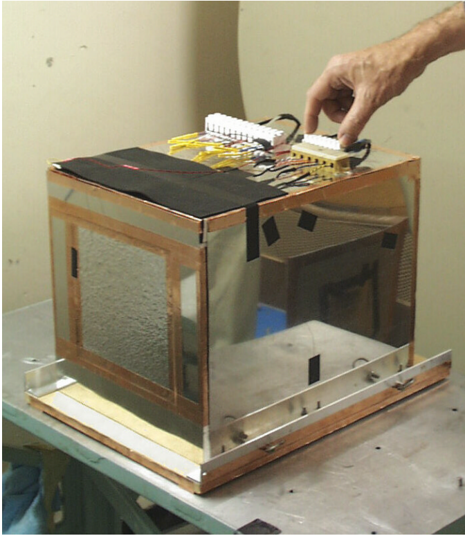
Figure 4: Calorimeter body showing the inner shielding layer.
