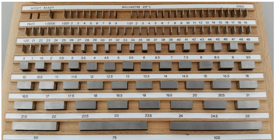
Figure 5. A gauge block set contains gauge blocks of different sizes.
