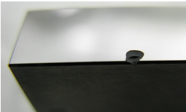
Figure 3. Chipped measuring face on a gauge block.
