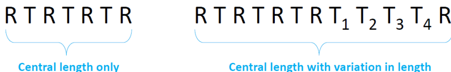
Figure 12. Sequence of measurements in gauge block calibration.
