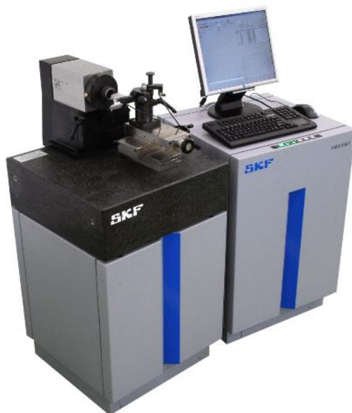
Figure 8. A waviness measurement machine with inductive sensors. Reproduced with permission from SKF [18].
