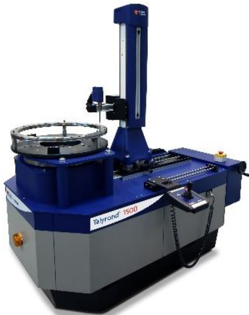
Figure 7. An example of a large roundness measurement machine. Reproduced with permission from Taylor Hobson Ltd [17].
