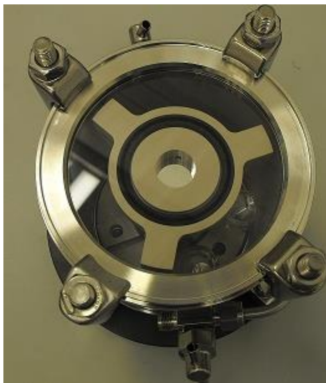
Figure 3. NPL inert gas/vacuum compatible storage vessel used in this study.
