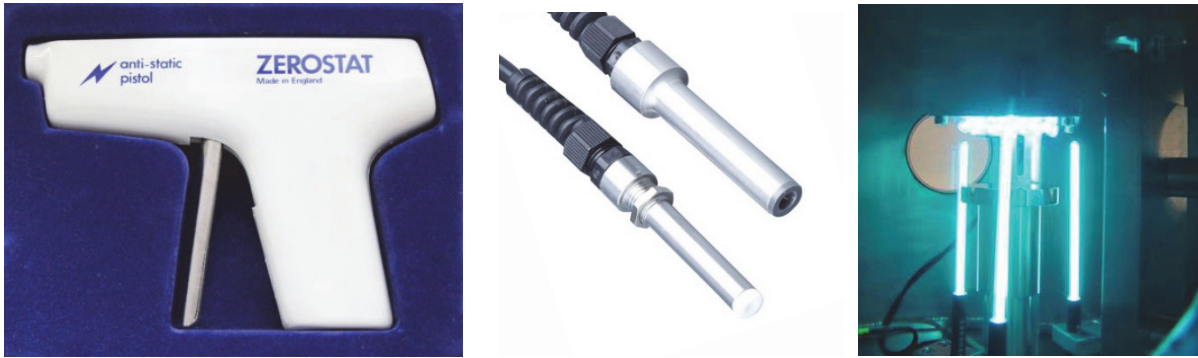
Figure 7: Static charge removal equipment (Zerostat anti-static gun, Fraser ion source, UV lamp)
