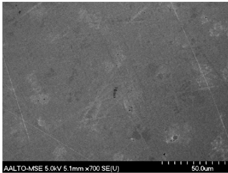
Figure 5. SEM micrograph at \times 700 magnification of gold-electroplated copper surface produced by Häfner.
