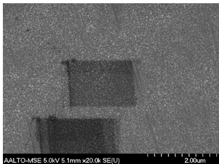
Figure 6. SEM micrograph at \times 20,000 magnification of gold-electroplated copper surface produced by Häfner.
