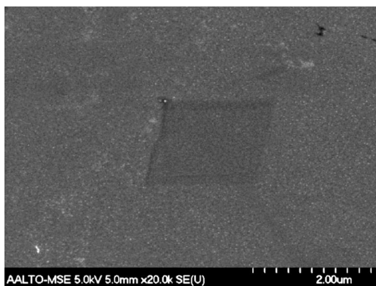
Figure 11. SEM micrograph at \times 20,000 magnification of rhodium-electroplated copper surface produced by Häfner.
