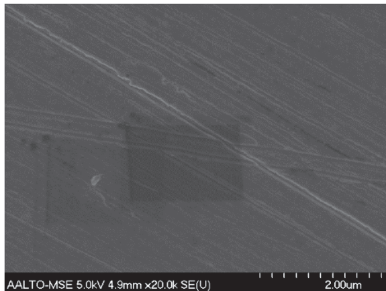
Figure 5. SEM micrograph at \times 20,000 magnification of platinum-iridium sample surface.
