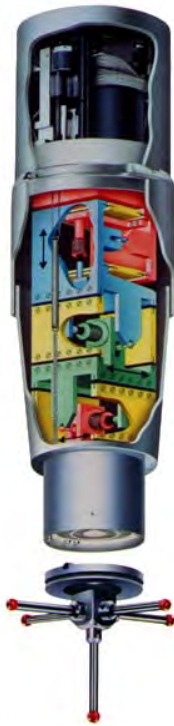
Figure 14 An exploded diagram of an analogue probe head (©Zeiss)
