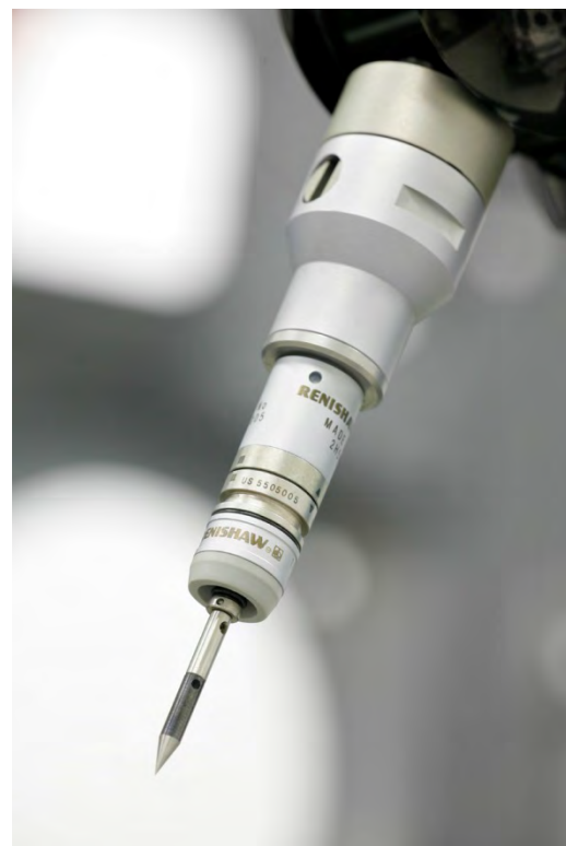
Figure 31 An application of a pointer stylus (© Renishaw plc 2014)
