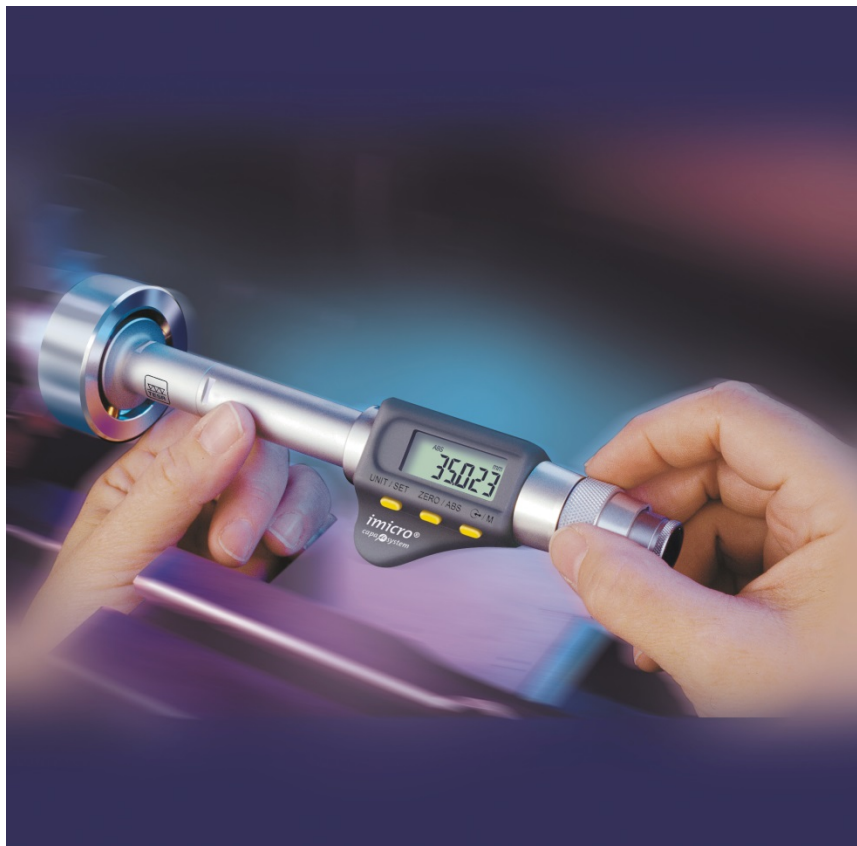
Figure 70 A three point inside micrometer in use (courtesy Tesa Group)
