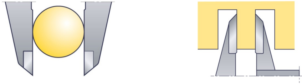
Figure 10 External measurement (courtesy Tesa Group).
