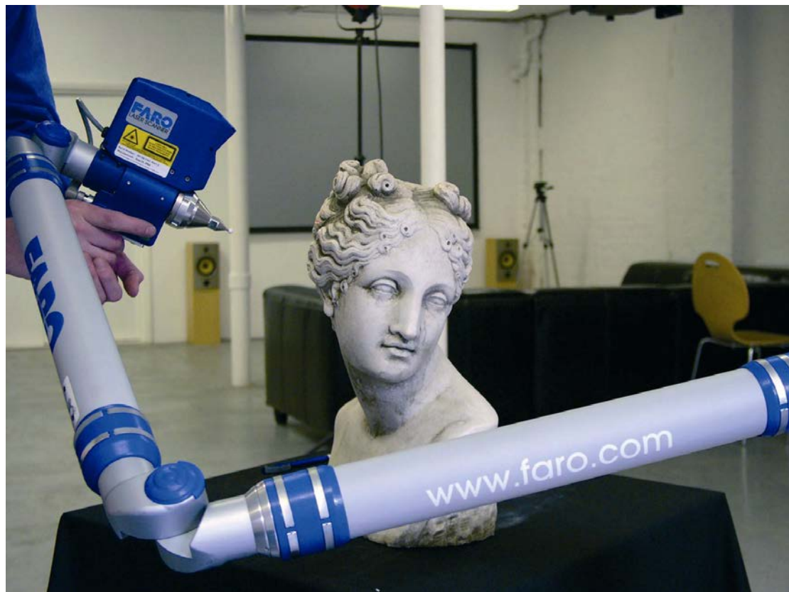
Figure 76 A laser scanner in use with an articulated arm (courtesy Faro)
