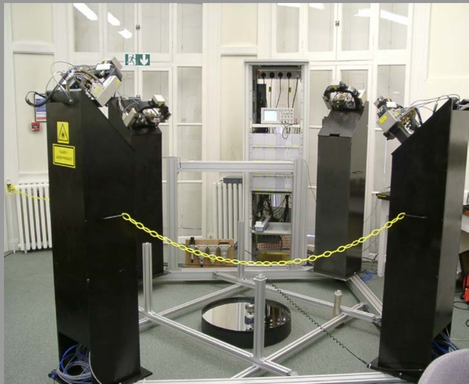
Figure 23 Multilateration in action
