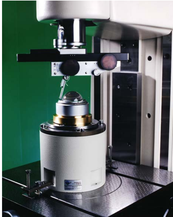
Figure 32 A hemisphere being measured by the multi-step method
