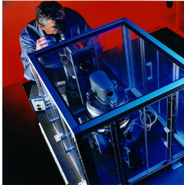
Figure 39 Shielding the equipment from draughts
