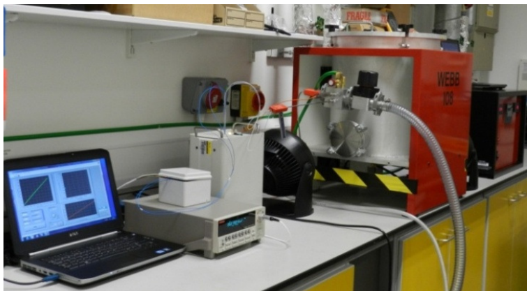
Figure 3: Photograph of the ‘breadboard’ for testing the self-validating thermocouples. Left to right: PC, digital nanovoltmeter (with connection box on top), automatic ice point, high temperature furnace.
