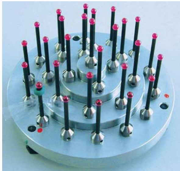
Figure 28. Zeiss calibration reference sphere [134]
