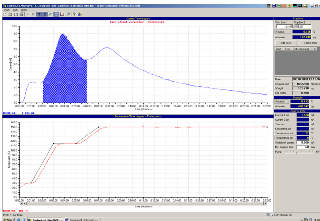
Figure 2: “Capillary water” fraction resolved from results of coulometric analysis of evolved vapour of polyethylene terephthalate (PET) sample.
