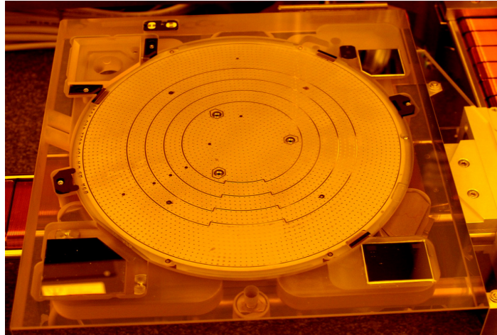
Figure 25 Nobel Metal Stepper at MiPlaza – stepper fixture.
