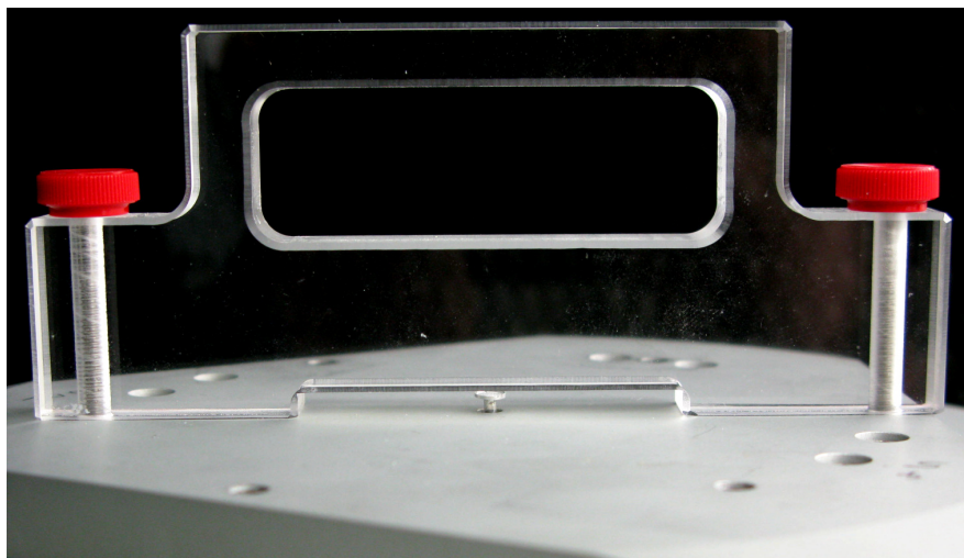
Figure 48 Metrology at NPL – Low Force Balance. Multiple fixtures can be easily attached above the weighing platen.
