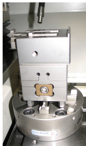
Figure 35 ULTRA Lab at Tekniker – micro-milling fixture.
