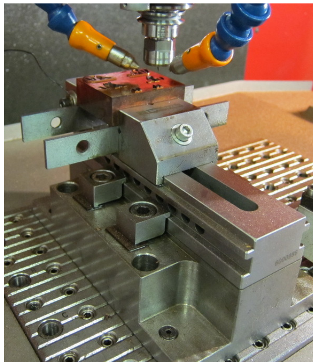
Figure 7 Mastermaking at Cardiff University – micro precision milling using a vice fixture. Alignment is achieved by using a touch probe.
