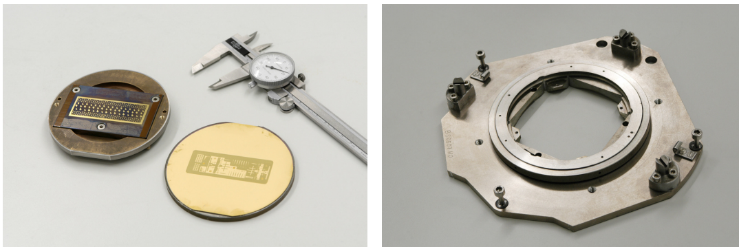
Figure 17 Direct X-ray lithography at KIT – a round mask and a rectangular mask in an adapter (left) and the mask fixture (right).
