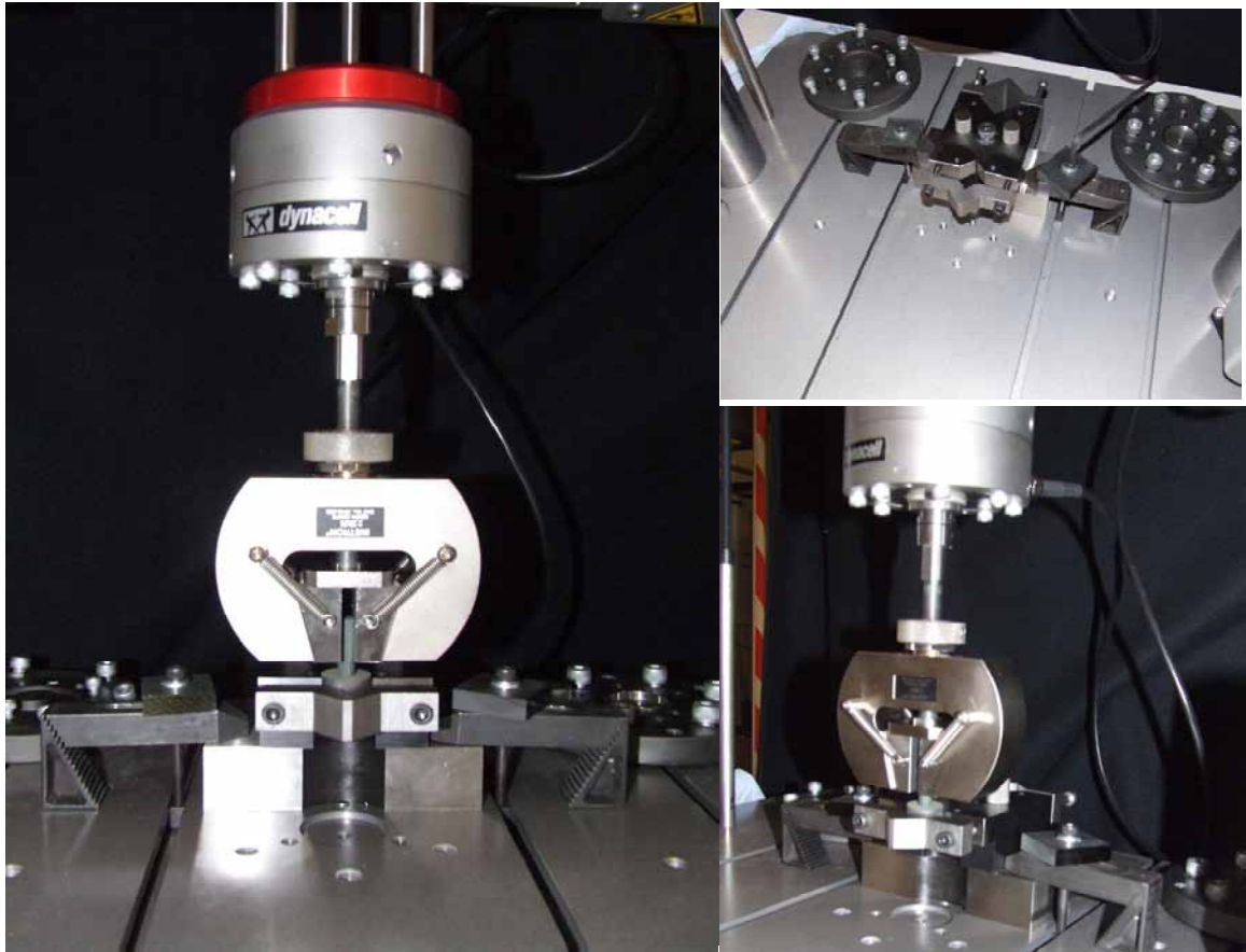
Figure 5 Photo showing the gripping method used for the pin and collar samples in the ElcetroPuls tensile tester.
