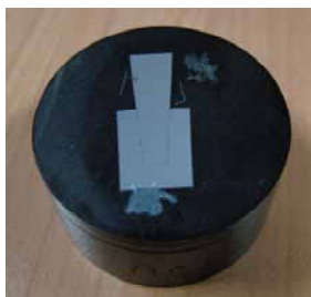
Figure 2 Stainless steel pin and collar sample used to assess the feasibility of this specimen design. Micrograph shows the oxide formed on the bottom of the pin at the two edges and the centre.
