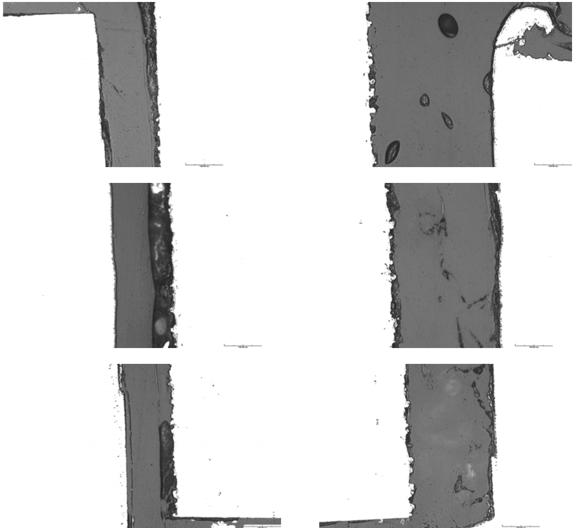
Figure A8 AARC004 – IN740 Pin in an IN617 Collar, 3000h at 750°C.
