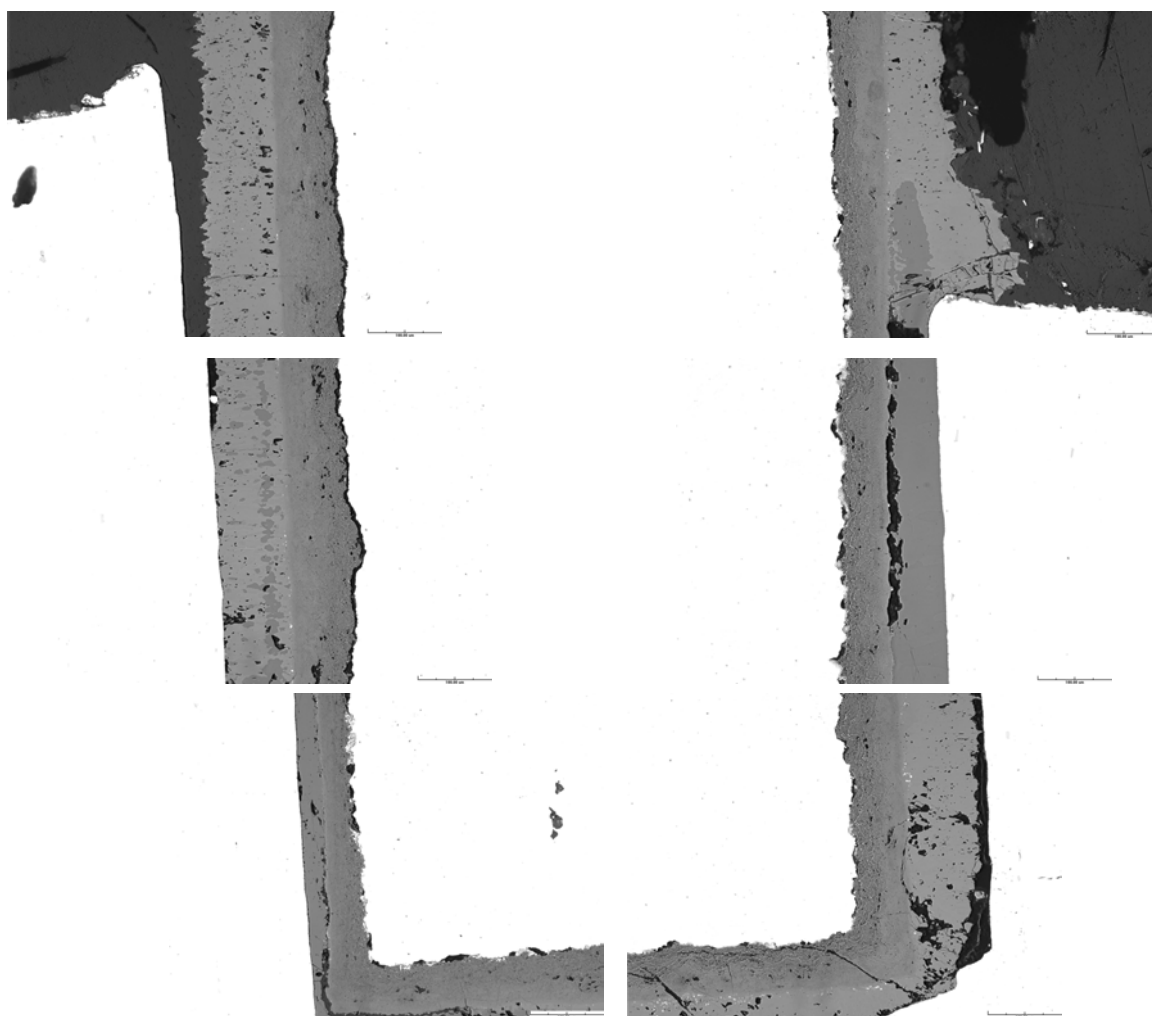
Figure A14 AARE002 – P92 Pin in an IN617 Collar, 1000h at 650°C.
