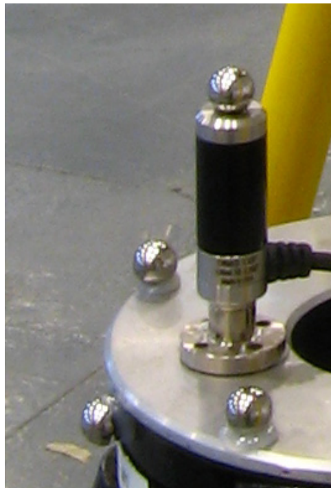
Figure 9. Receiver monument comprising four tooling balls and an iGPS receiver.
