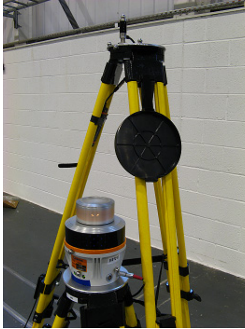
Figure 8. Close up of a transmitter/receiver monument pair.
