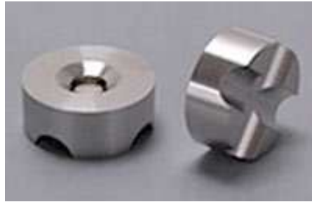
Figure 4 a pair of ½ inch drift nests.
