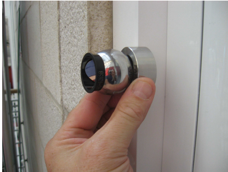
Figure 10 The edge tool being used to measure a doorframe.
