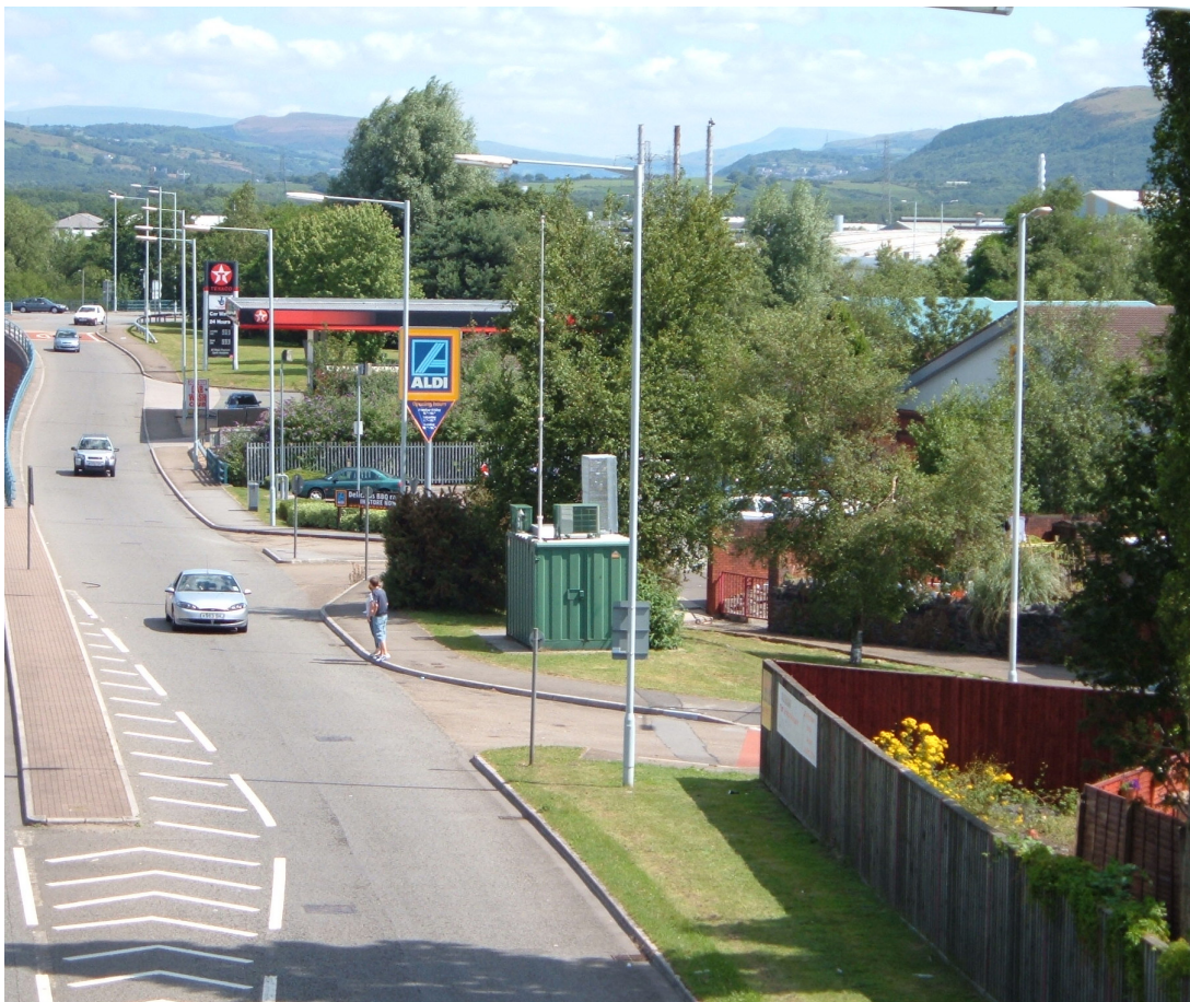
Image 2. The new Network site at Swansea Morriston. The Partisol 2000 sampler is located in the tall cage on top of the green monitoring cabin in the centre of the picture.
