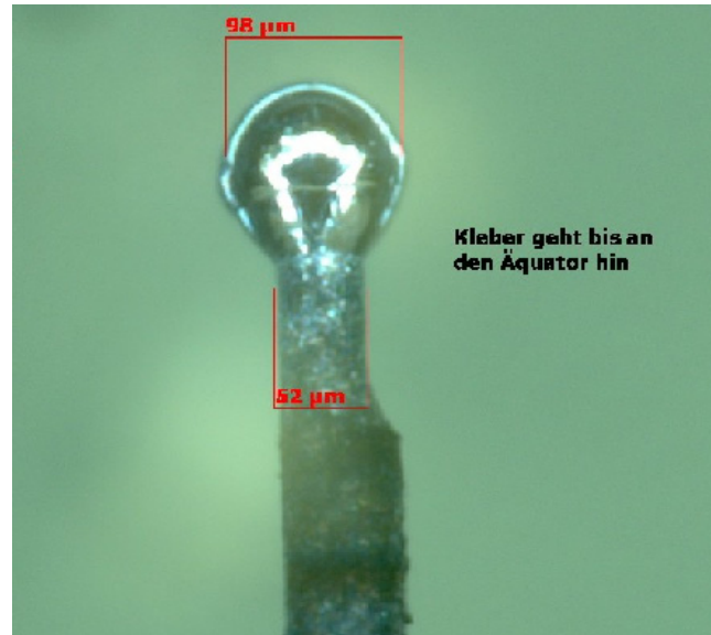
Figure 17: Measuring microscope image of NPL/Zeiss microprobe NPL-4 showing the probe tip.
