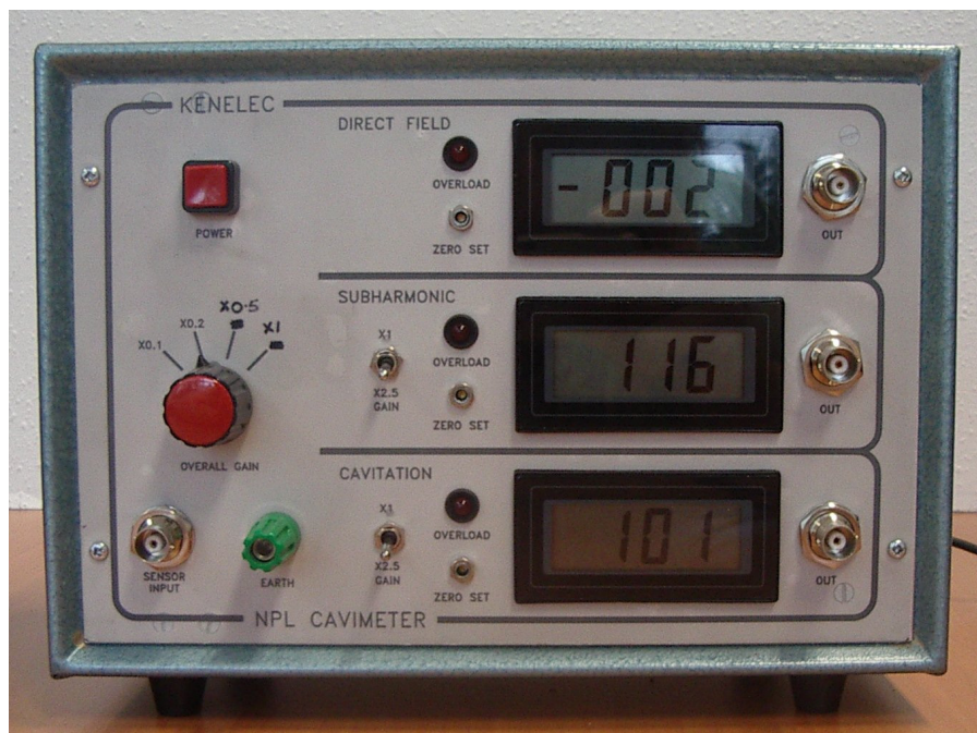
Figure 5.3: Breadboard prototype of Cavimeter
