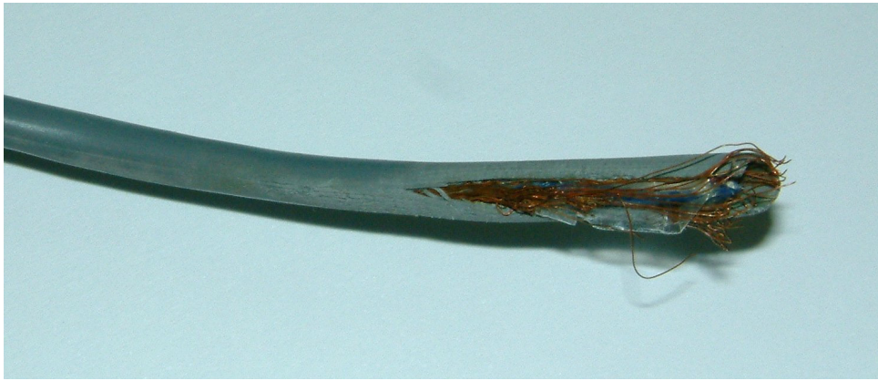
Figure 4.6: Cavitation erosion on cable from sensor JIP 30_01
