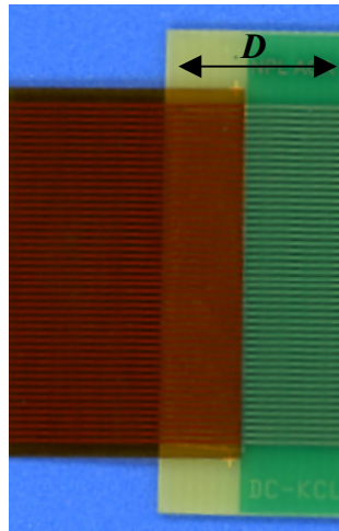
Figure 4: Interconnect under test joining rigid and flexible PCBs. The join occurs at a distance D along the line
