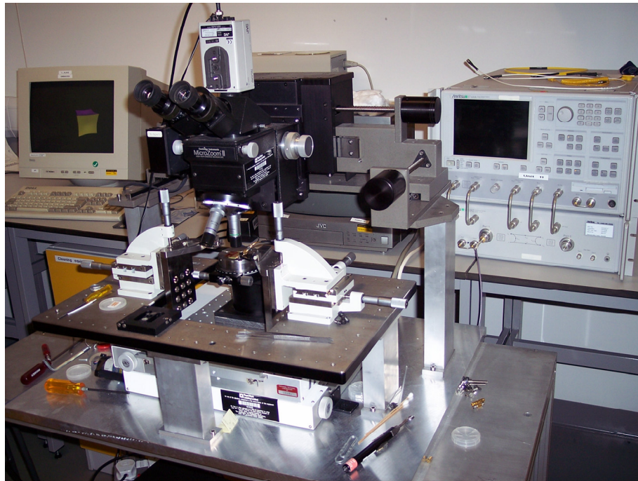
Figure 7: The complete measurement system: VNA (right-hand-side); probe station (centre); and, probe/test coupon (immediately below the microscope)
