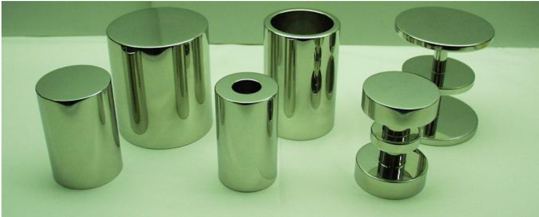
Figure 4: Large (back) and small (front) air density artefacts. From left to right: hollow shape, tube shape and bobbin shape
