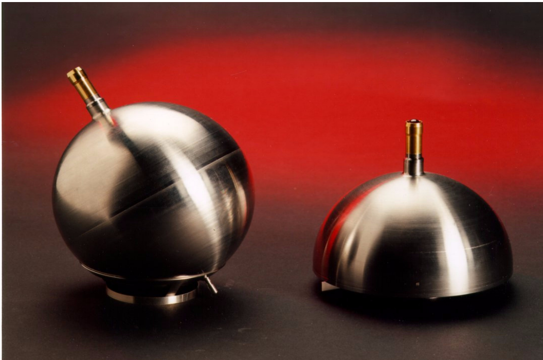
Figure 2: Mk I air density artefacts manufactured at NPL in 1994
