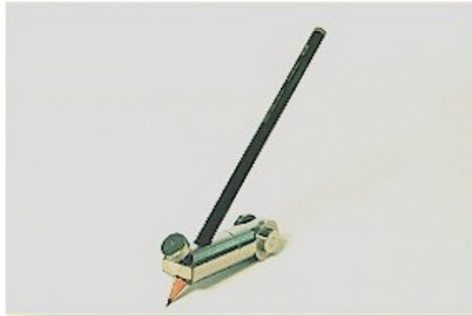
Figure 3 : Pencil hardness test
