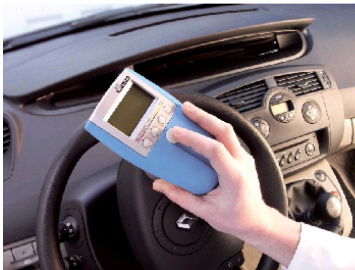
Figure 4 : Typical handheld Gloss Meter (source: BYK Gardner)
