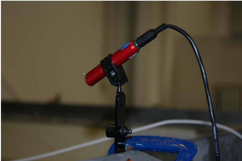
Fig. 3.3: Laser alignment module and adjustable mounting bracket clamped to the side of the tank.
