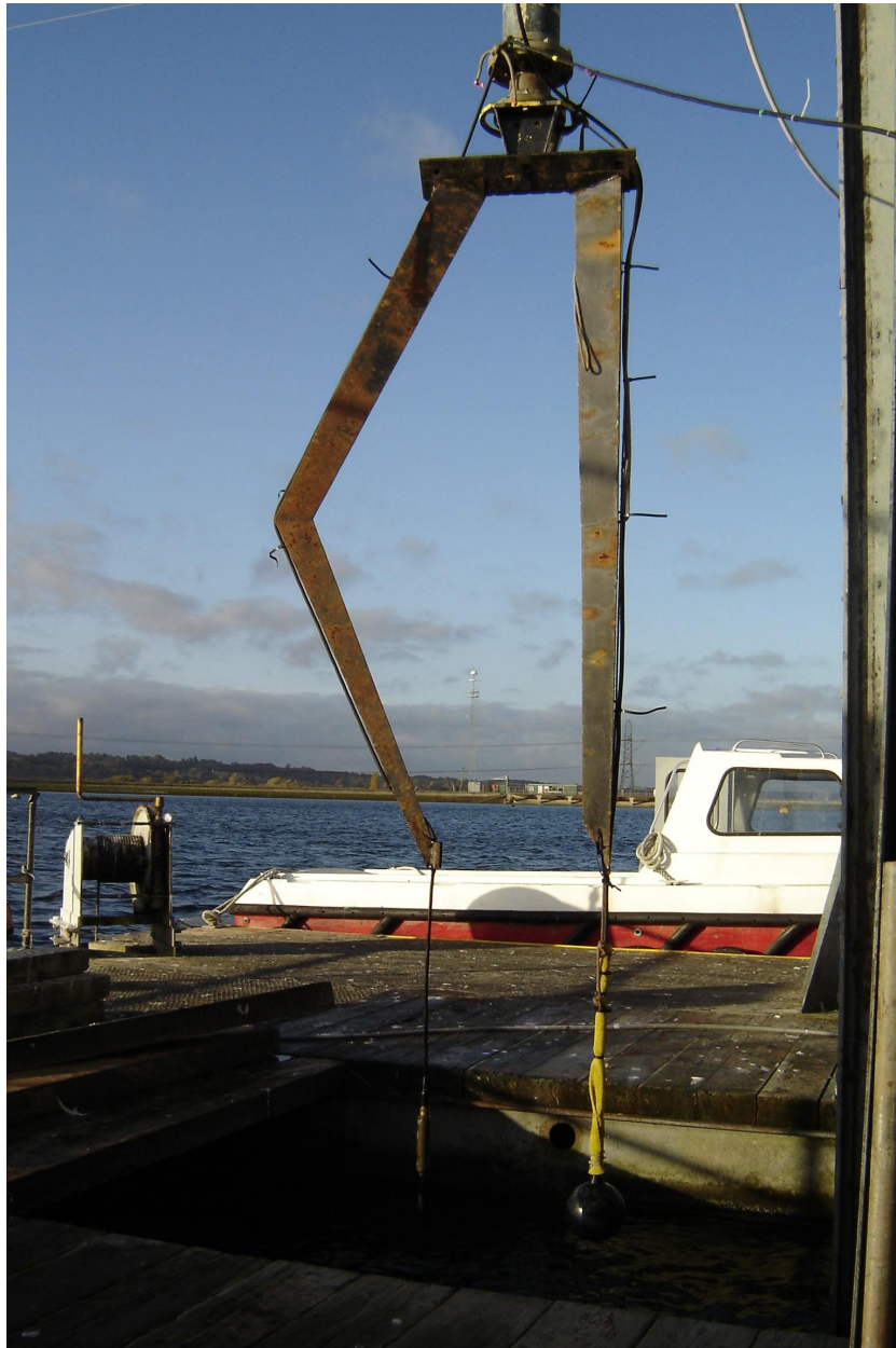
Fig 2.3 Mounting arrangement used for low frequency calibrations
