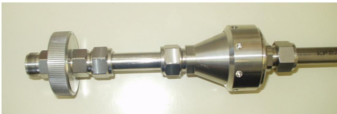
Figure 2. Example of the configuration of a filter holder under test (in this case an Apex filter holder in line with a Tecora filter holder, with a PTFE filter).
