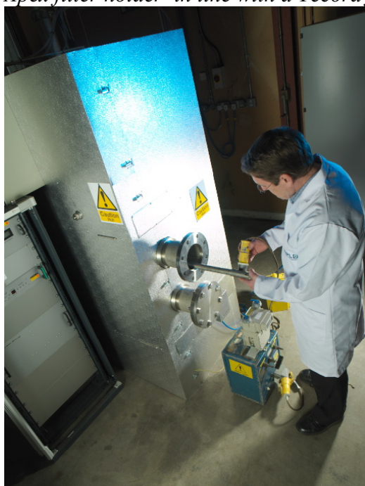
Figure 2. Example of the configuration of a filter holder under test (in this case an Apex filter holder in line with a Tecora filter holder, with a PTFE filter).
