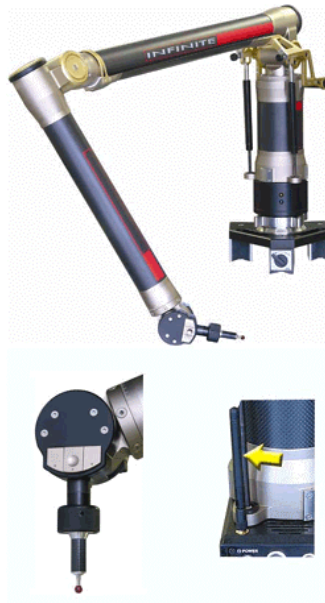
Figure 8: Example of Cimcore articulating arm promoted at Inspex 2005 (Courtesy of Europac [77])
