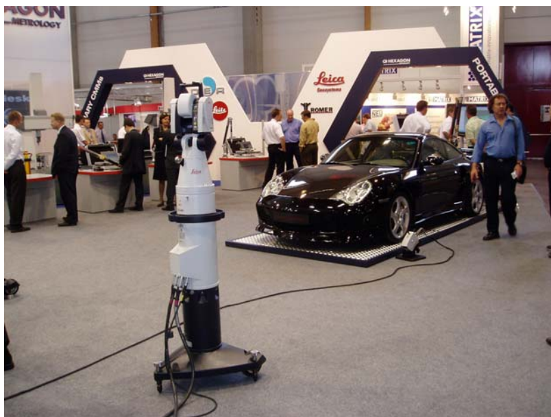
Figure 6: Leica laser tracker in operation at Control-2006
