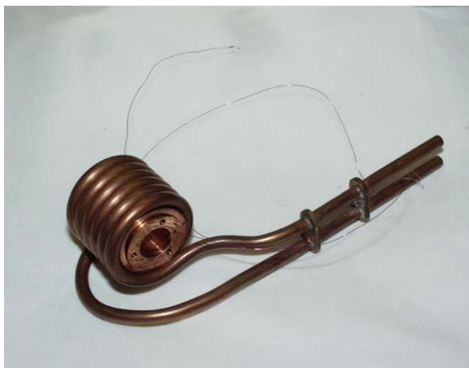
Figure 8. Cooling coil surrounding Maxwell pair coil assembly.
