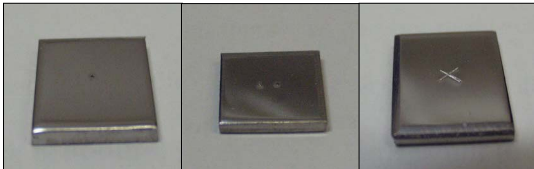
Figure 3: Stainless steel coupons stamped with a single dot (left), double dot (centre) and an X (right)
