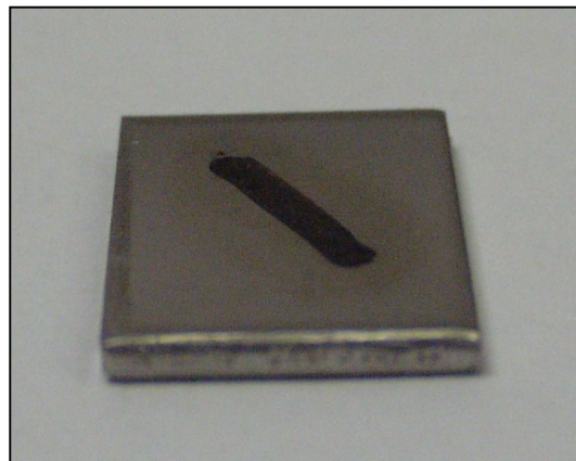
Figure 5: An acid etched stainless steel test coupon
