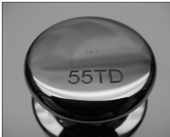
Figure 1: The top of an OIML shape 1 kg stainless steel weight with its identification '55TD' marked with a laser
