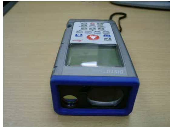
Figure 75 An ADM from the front
