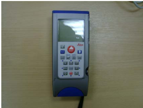
Figure 74 An absolute distance meter
