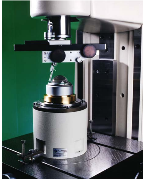
Figure 32 A hemisphere being measured by the multi-step method
