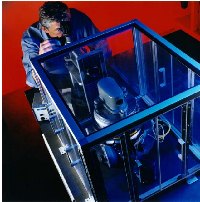
Figure 39 Shielding the equipment from draughts
