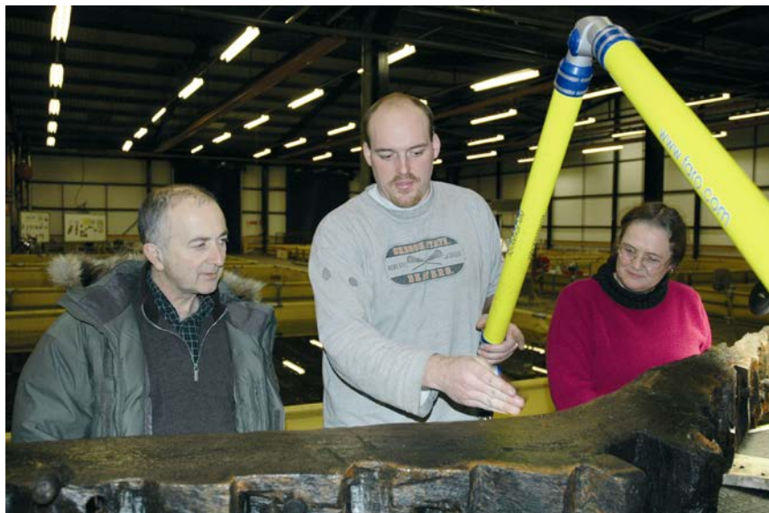
Figure 21 An articulated arm being used to measure the Newport Ship (Courtesy Faro UK and Newport Ship Project)
