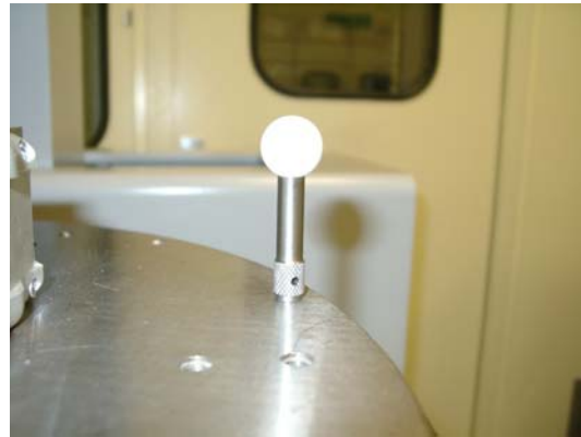
Figure 14 Attaching spheres allows repositioning to be used.
