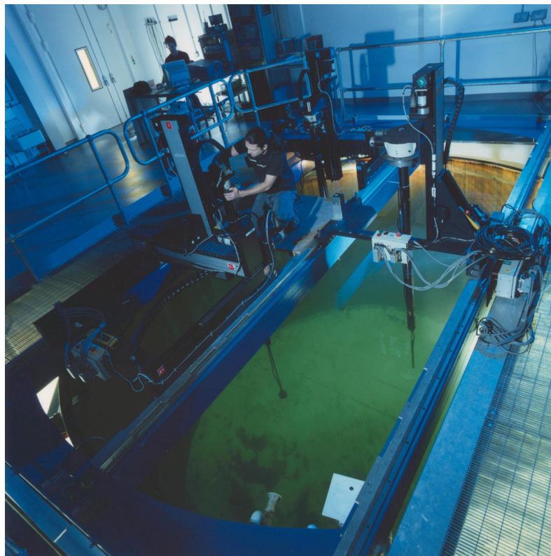
Figure 5.1 Photograph of the NPL large Open Tank Facility showing the carriages of the positioning system
