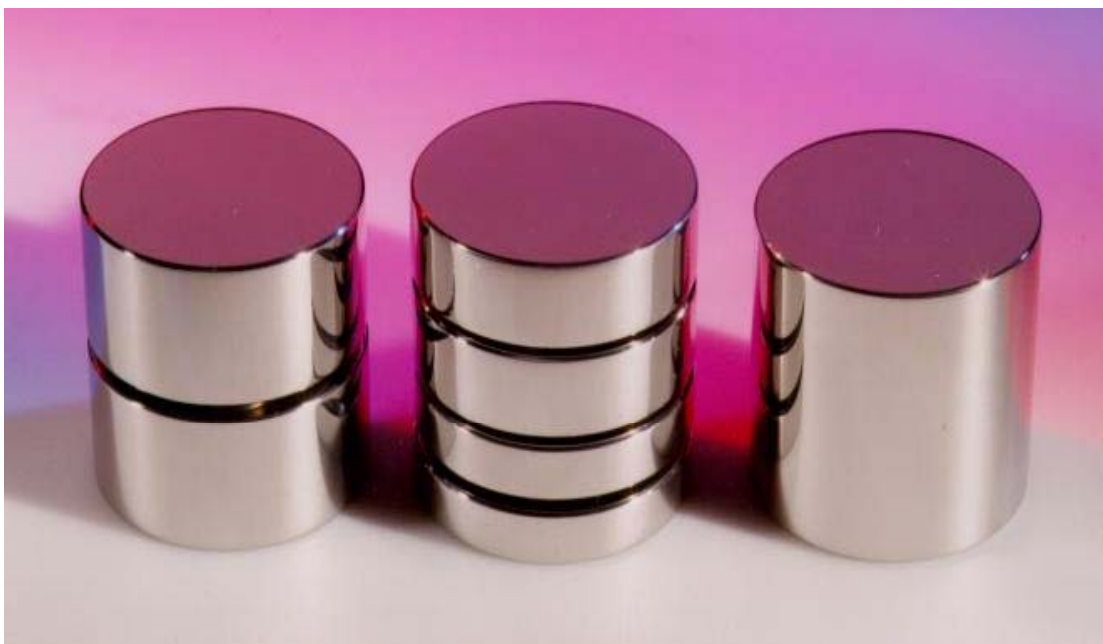
Figure 4: An assembled set of 1 kilogram weights of different surface areas designated 500s, 2/300s and 1000(2)
