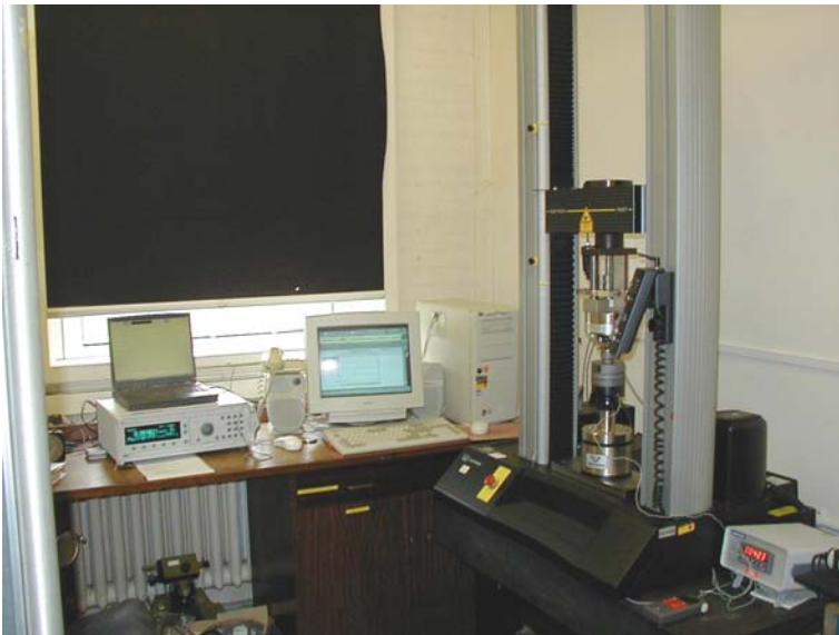
Figure 6 NPL 30 kN hardness standard machine
