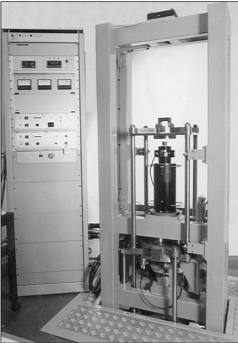
Figure 1 The 20 kN deadweight force standard machine
