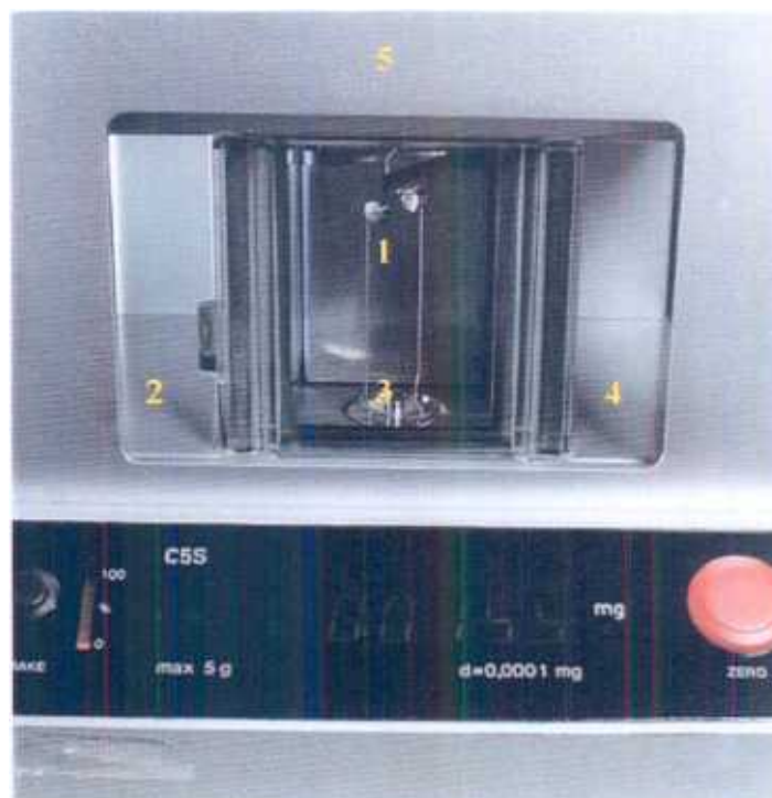
Figure 1: C5S with relative position of thermistor probes
