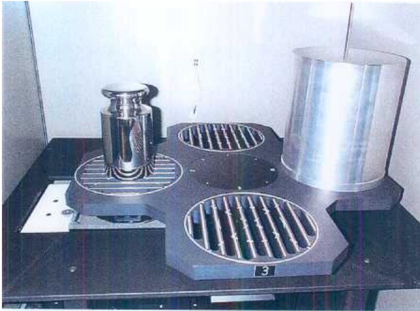
Figure 7: Aluminium cylindrical cans used on the C10000S as individual draft shields
