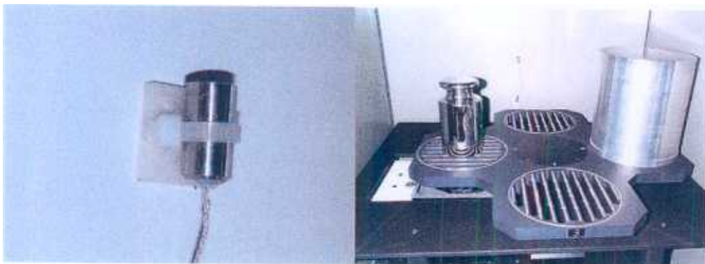
Figure 1: Thermistor probe and its siting in a balance enclosure
