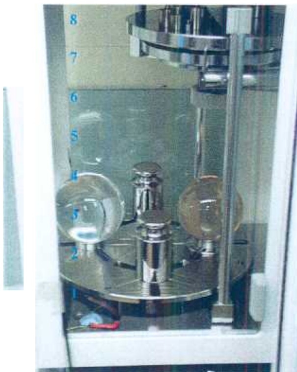
Figure 4: AT10005 with relative position of thermistor probes.
