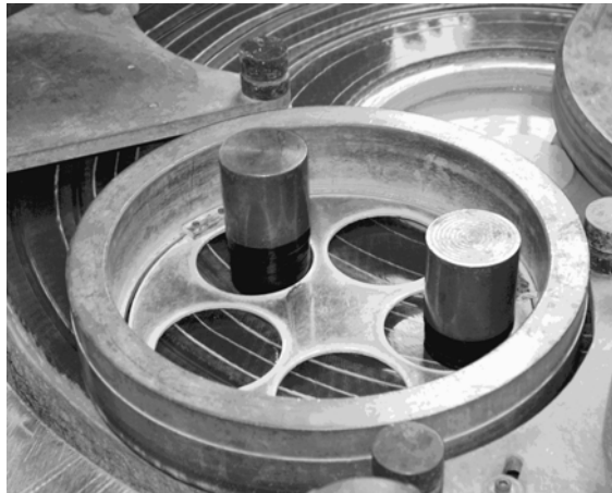
Figure 2–1. Two artefacts being polished on a lapping machine in the NPL Optical Workshop
