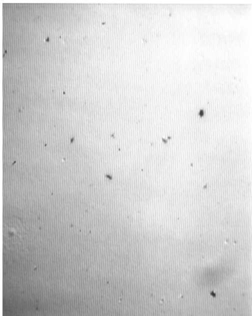
Figure 5 The same sample as in figure 4 after blowing with compressed air (left) and after cleaning with ethanol (right).
