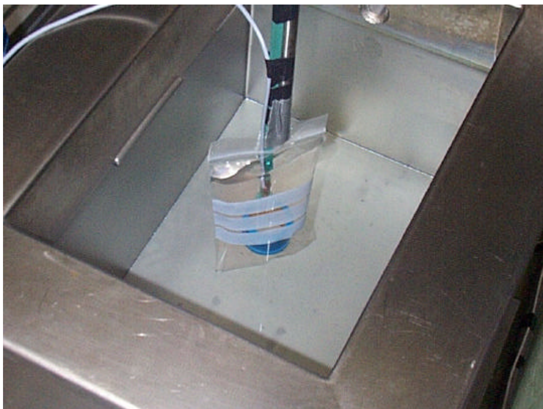
Figure 6.20: PCS-11 located inside polyethylene sample bag in reference vessel
