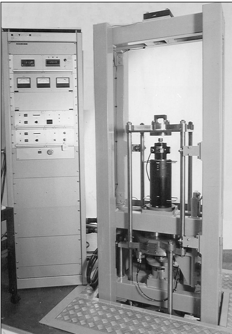
Figure 4 20 kN deadweight force standard machine
