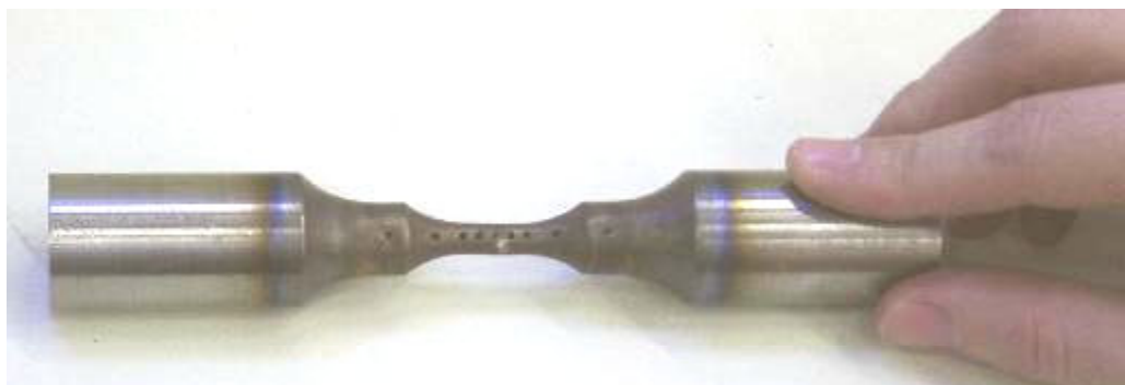
Figure 21 Temperature profile calibration testpiece with holes drilled for calibration thermocouples, as used at Sheffield University.
