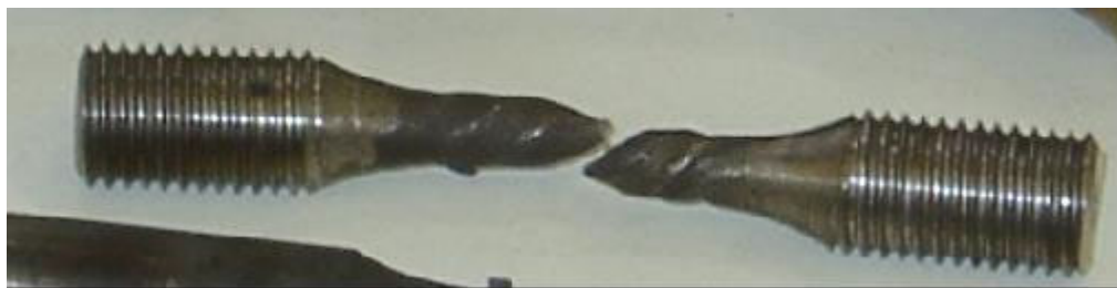
Fig 23 Helical ridges after testing.
