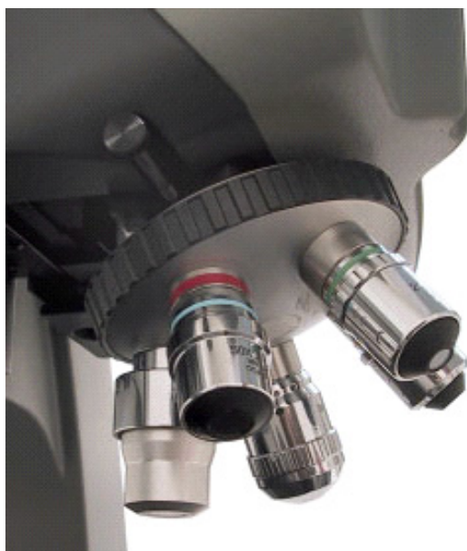
(a) Manual turret holding five objective lenses
