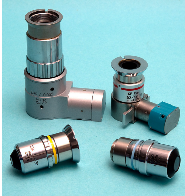
Figure 17 Four lenses used on a CSI instrument. Clockwise from top left: 2× Michelson, 5× Michelson, 20× Mirau and 10× Mirau
