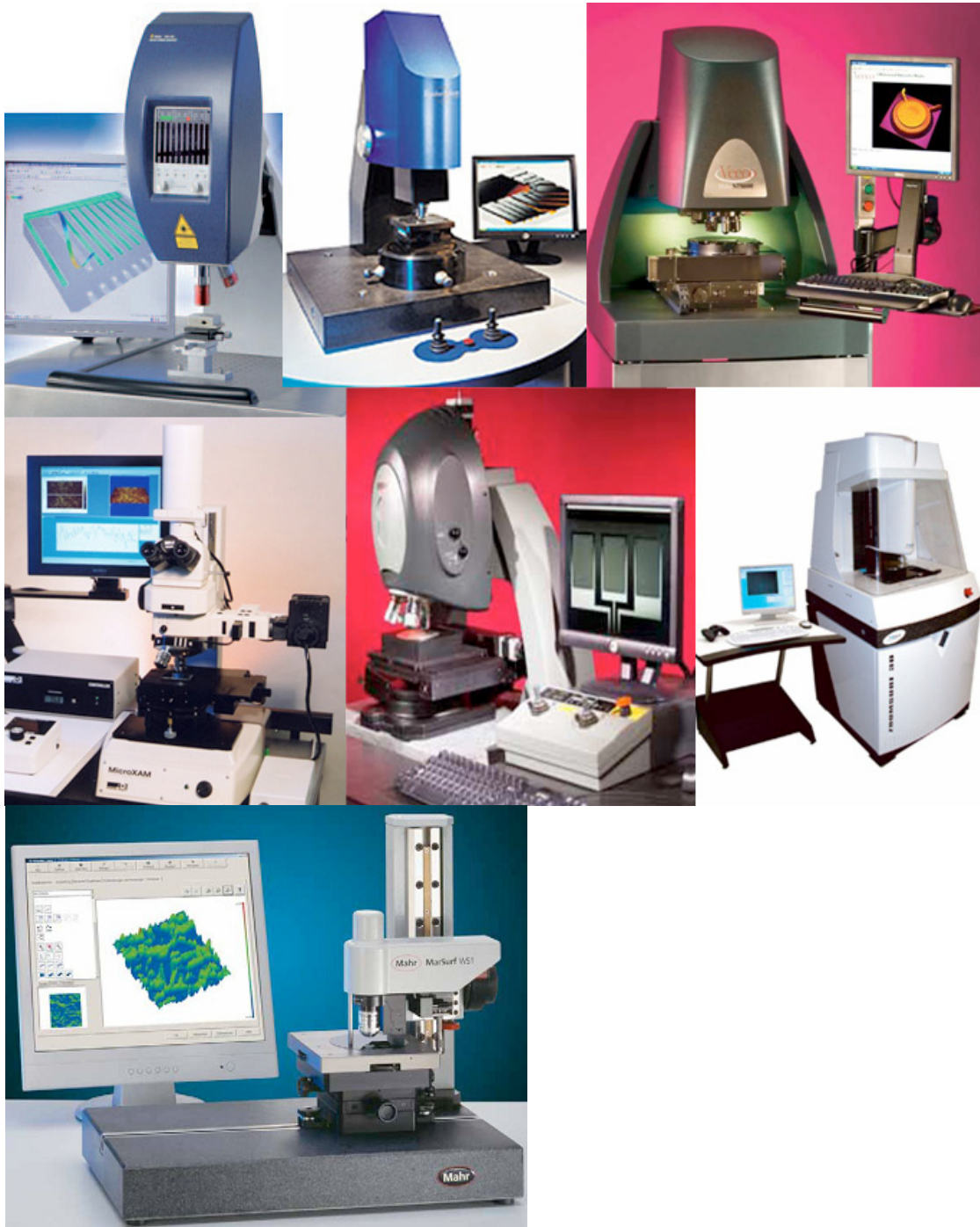
Figure 6 A selection of commercially available CSIs. Clockwise from bottom left: Mahr, Phase Shift, Polytec, Taylor Hobson, Veeco, Fogale and Zygo
