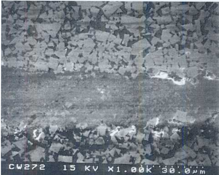
Figure 29 Scanning electron micrographs of low load scratch tests on CWC20C hardmetal, a) single pass with 200 \mu\text{m} indenter, b) 5 passes with 200 \mu\text{m} indenter, c) 50 passes with 200 \mu\text{m} indenter, d) 100 passes with 200 \mu\text{m} indenter, e) 100 passes with 200 \mu\text{m} indenter, f) 100 passes with 200 \mu\text{m} indenter, g) 100 passes with 200 \mu\text{m} indenter.
