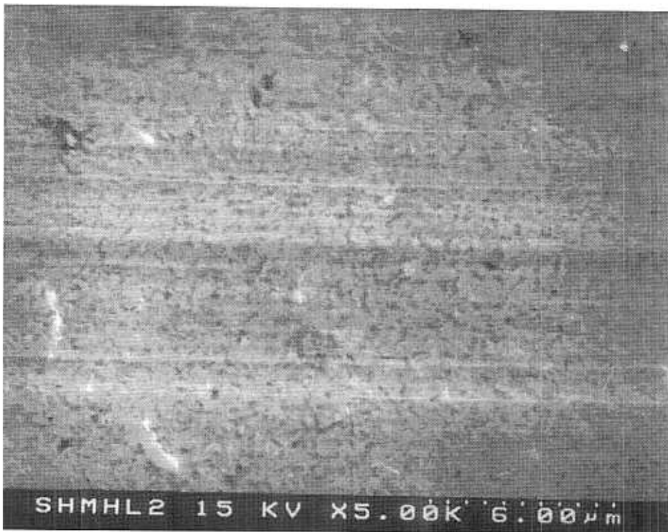
Figure 10, Scanning electron micrographs on hardmetals scratched in high load tests, a) SHMUF, b) SHMUF, c) CW20C, d) CWC20C.
