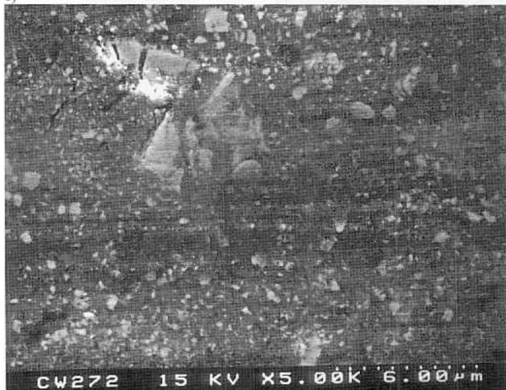
Figure 29 Scanning electron micrographs of low load scratch tests on CWC20C hardmetal, a) single pass with 200 \mu\text{m} indenter, b) 5 passes with 200 \mu\text{m} indenter, c) 50 passes with 200 \mu\text{m} indenter, d) 100 passes with 200 \mu\text{m} indenter, e) 100 passes with 200 \mu\text{m} indenter, f) 100 passes with 200 \mu\text{m} indenter, g) 100 passes with 200 \mu\text{m} indenter.
