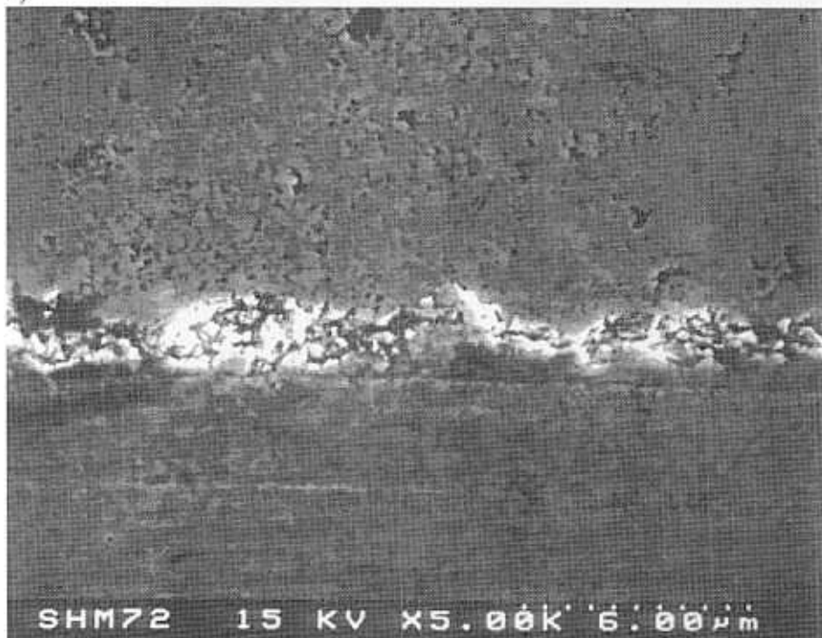
Figure 30, Scanning electron micrographs of low load scratch tests on SHMUF hardmetal, a) single pass with 200 \mu\text{m} indenter, b) 10 passes with 200 \mu\text{m} indenter, c) 50 passes with 200 \mu\text{m} indenter, d) 10 passes with 50 \mu\text{m} indenter, e) 50 passes with 200 \mu\text{m} indenter, f) 100 passes with 200 \mu\text{m} indenter.
