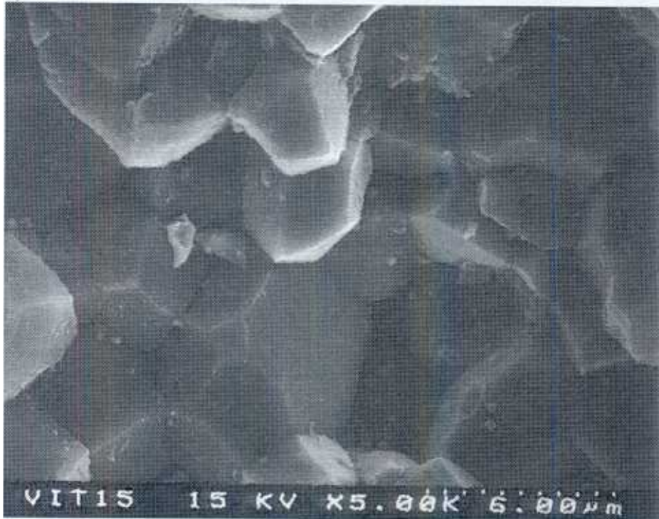
Figure 33, Scanning electron micrographs of low load scratch tests on Vitox ceramic, a) single pass with 50 \mu\text{m} indenter, b) single pass with 50 \mu\text{m} indenter, c) 10 passes with 50 \mu\text{m} indenter, d) 10 passes with 50 \mu\text{m} indenter, e) 50 passes with 50 \mu\text{m} indenter, f) 100 passes with 50 \mu\text{m} indenter, g) 5 passes with 200 \mu\text{m} indenter, h) 20 passes with 200 \mu\text{m} indenter, i) 50 passes with 200 \mu\text{m} indenter, j) 100 passes with 200 \mu\text{m} indenter.
