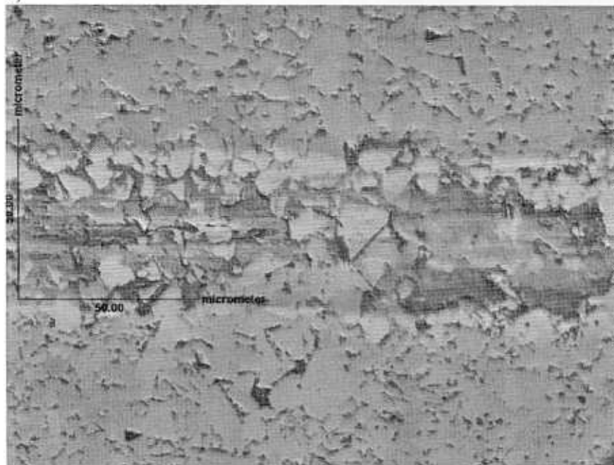
Figure 22, Low Load Scratches for a) TC222 hardmetal with a 200 \mu\text{m} indenter and a single pass, b) TC222 hardmetal with a 200 \mu\text{m} indenter and 100 passes, c) SHMUF hardmetal with 200 \mu\text{m} indenter and a single pass, d) SHMUF hardmetal with a 200 \mu\text{m} indenter and two passes, e) SHMUF hardmetal with a 200 \mu\text{m} indenter and 100 passes.
