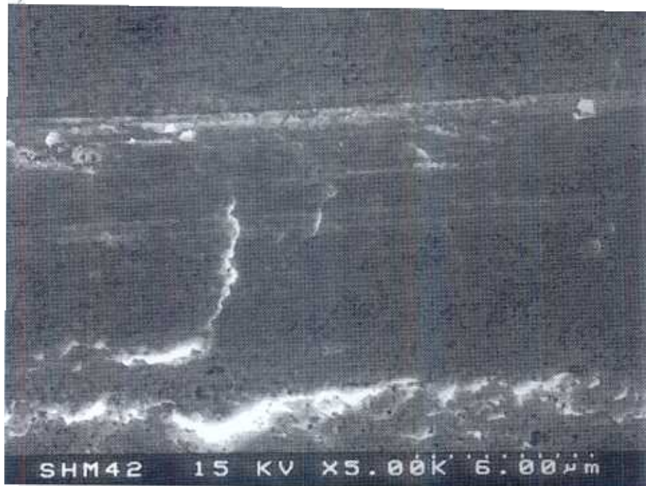
Figure 30, Scanning electron micrographs of low load scratch tests on SHMUF hardmetal, a) single pass with 200 \mu\text{m} indenter, b) 10 passes with 200 \mu\text{m} indenter, c) 50 passes with 200 \mu\text{m} indenter, d) 10 passes with 50 \mu\text{m} indenter, e) 50 passes with 200 \mu\text{m} indenter, f) 100 passes with 200 \mu\text{m} indenter.
