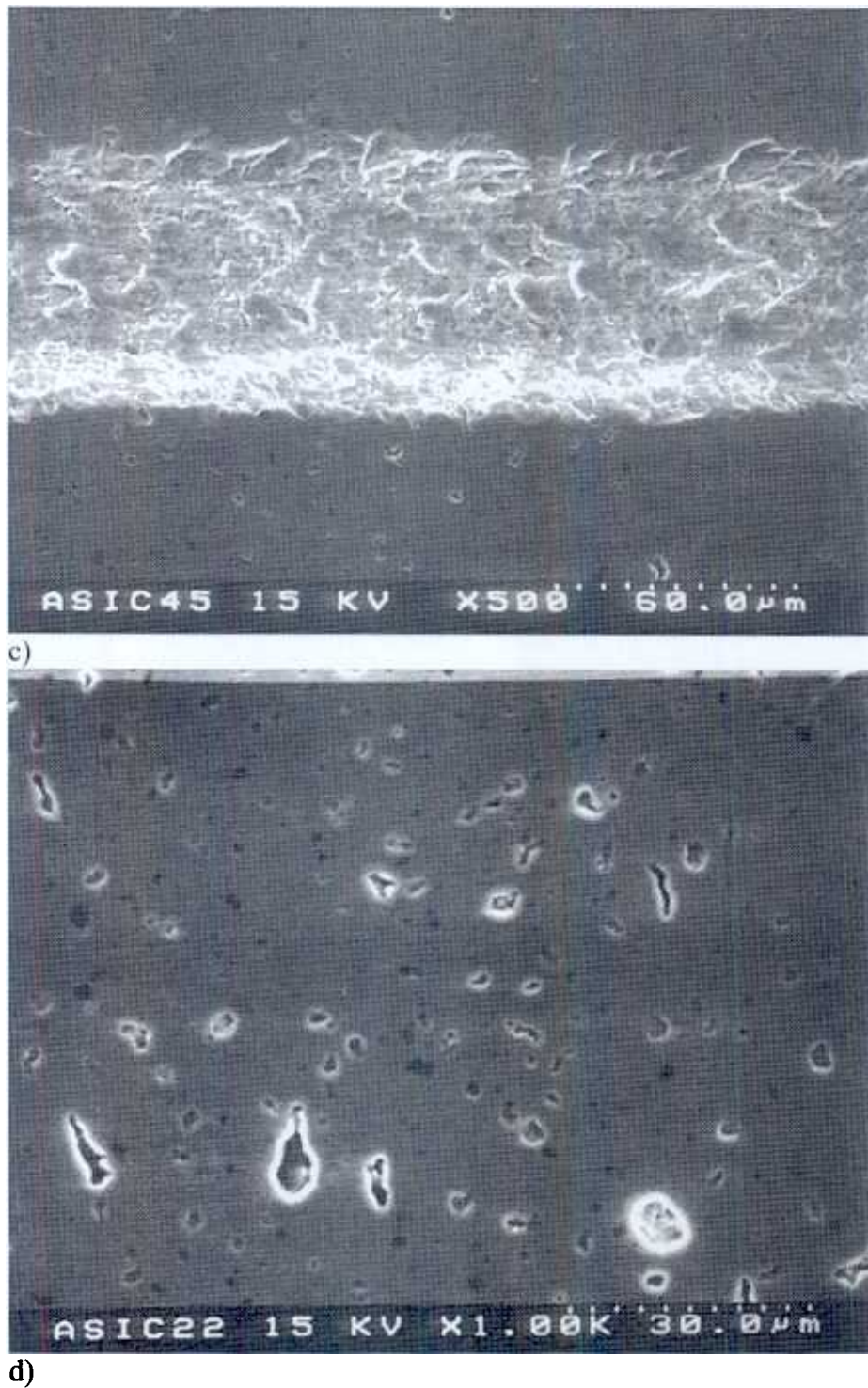
Figure 31, Scanning electron micrographs of low load scratch tests on \alpha -SiC ceramic, a) single pass with 50 \mu\text{m} indenter, b) 5 passes with 50 \mu\text{m} indenter, c) 10 passes with 50 \mu\text{m} indenter, d) 5 passes with 200 \mu\text{m} indenter, e) 20 passes with 200 \mu\text{m} indenter, f) 50 passes with 200 \mu\text{m} indenter, g) 100 passes with 200 \mu\text{m} indenter, h) 100 passes with 200 \mu\text{m} indenter, i) 100 passes with 200 \mu\text{m} indenter.
