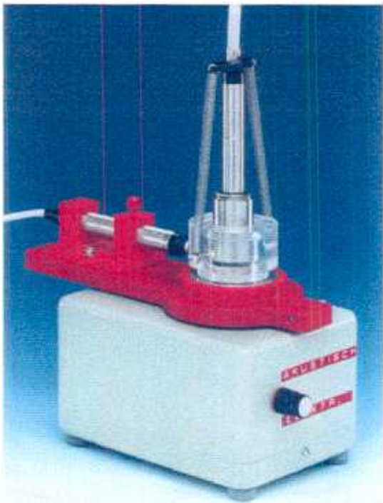
Figure 14 The coupler developed at PTB for WS1P microphones shown with microphones inserted.
