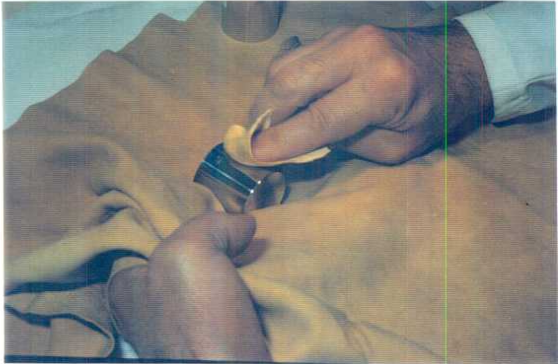
(a): by means of chamois leather moistened with a mixture of equal parts of ether and ethanol
