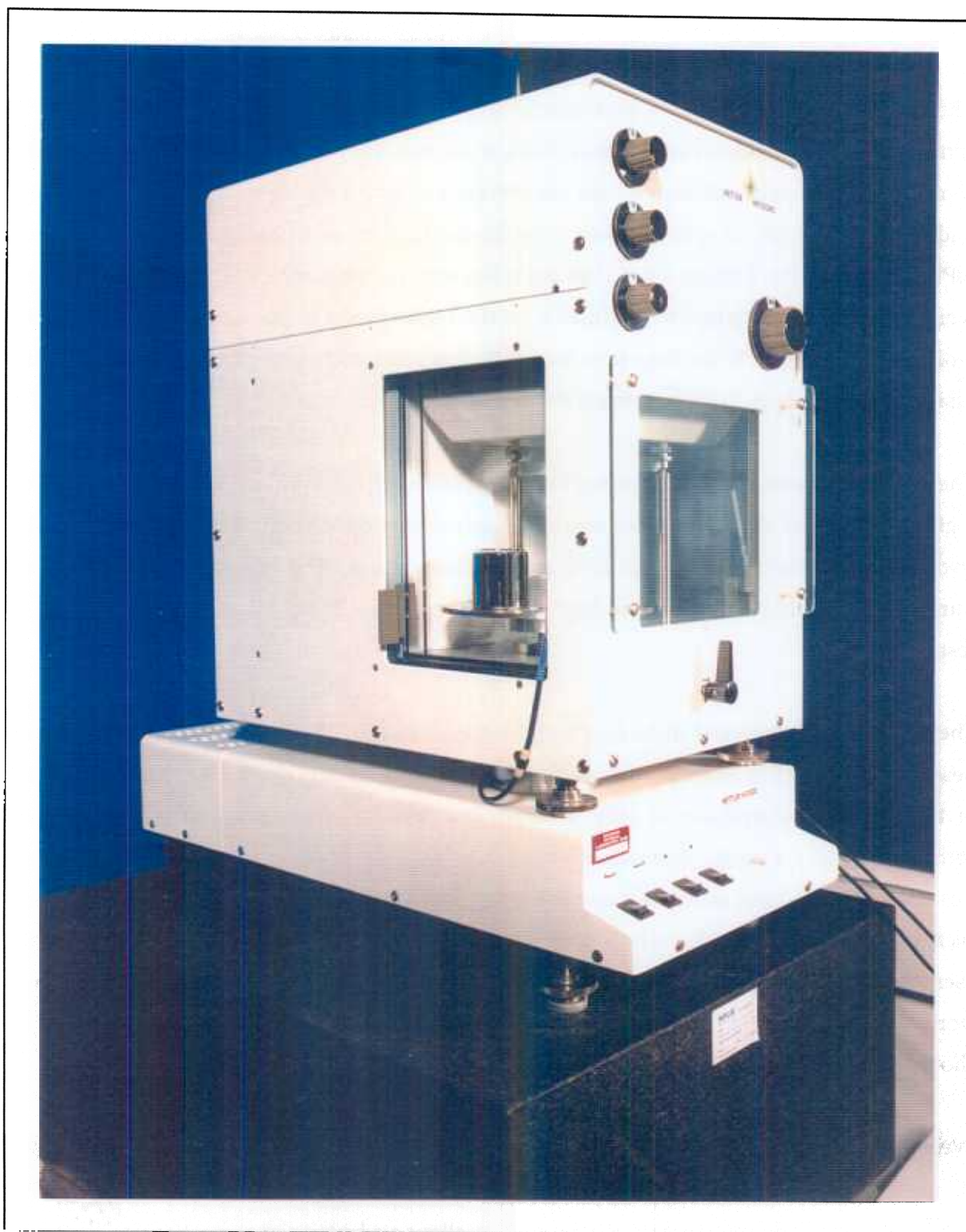
Figure 3.2 NPL's HK1000MC Force Balance in Ambient Conditions
