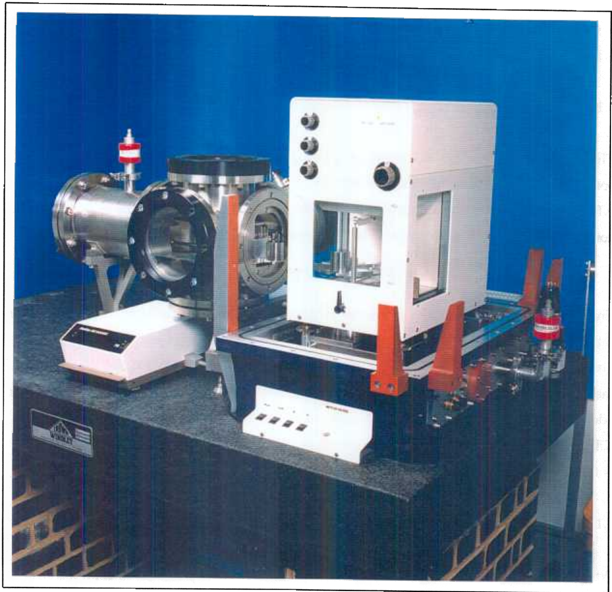
Figure 3.3.1: HK1000MC and Base of Vacuum Chamber
